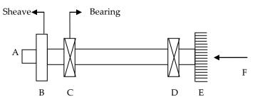
Fig. 2. Forces acting on the shaft
