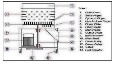
Fig.1. showing the drum style de-feathering machine with parts
